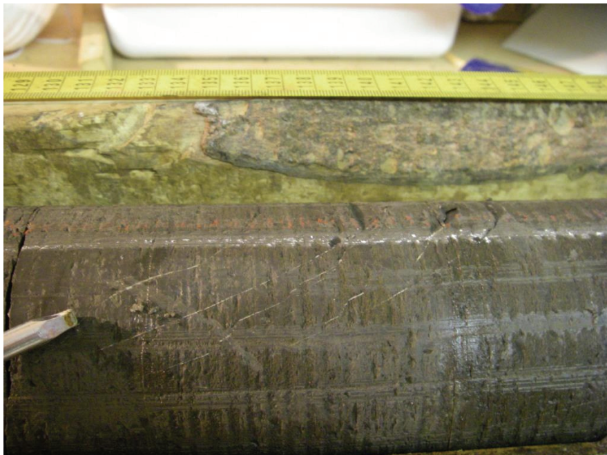
Figure 4.101: Closely Spaced, Inclined, Calcite-infilled Fractures at 638.5 mBGS in Blue Mountain Formation, DGR-3
