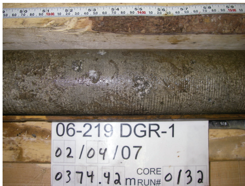
Figure 3.25: Core Photograph of Guelph Formation Porous Dolostone at 376 mBGS in DGR-1
