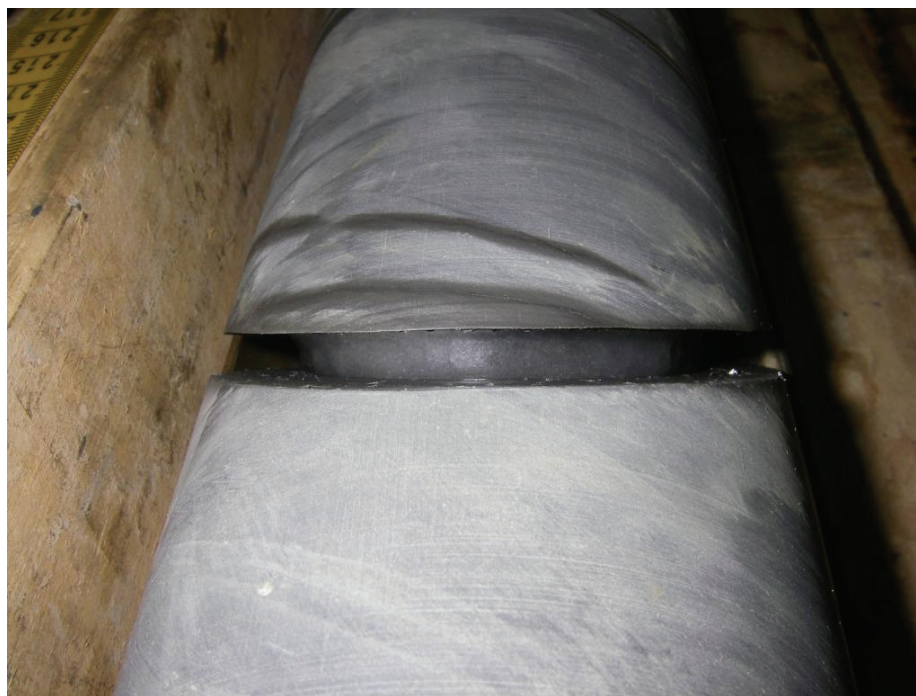
Figure 3.51: Partially Washed-out, White Halite Fracture Infill in the Lower Georgian Bay Formation Shale at 680.25 mLBS in DGR-6
