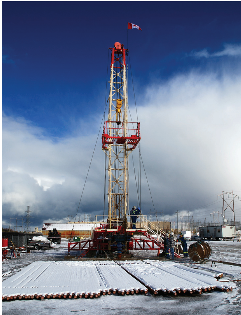
Figure 4.82: Straddle-packer Hydraulic Testing at DGR-4 Using Workover Rig and Drill Tubing
