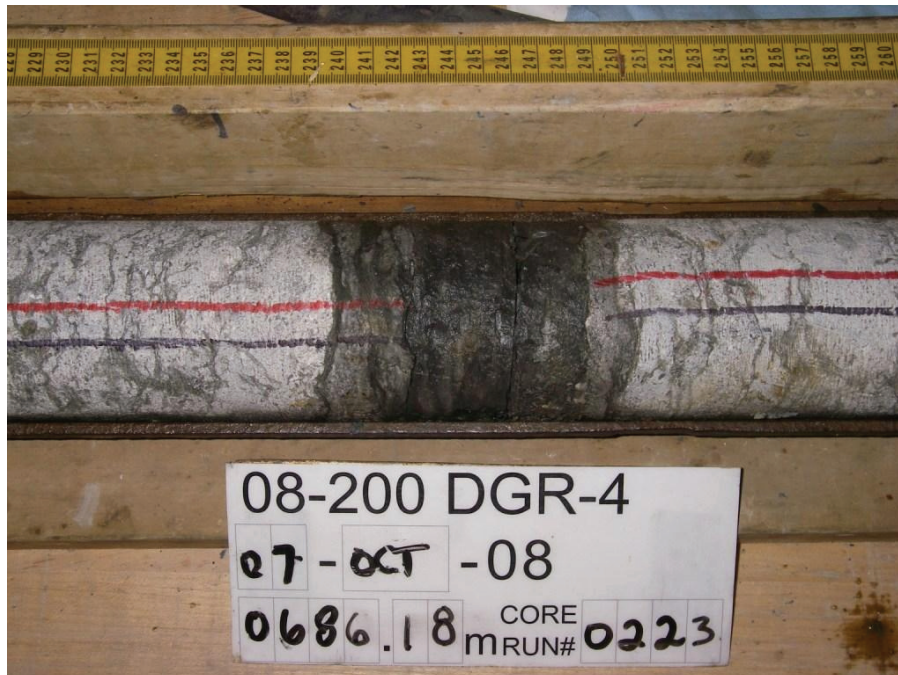
Figure 3.64: Fractured Fissile Shale Layer at a Depth of 688.6 mBGS in the Bottom of the Cobourg Formation, DGR-4
