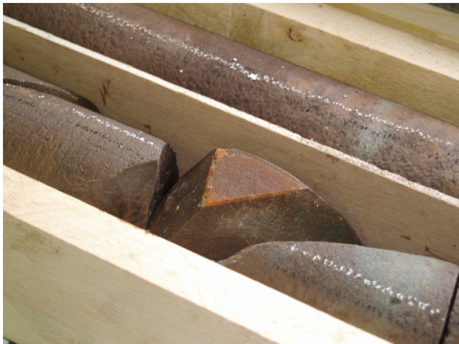
Figure 3.50: Orange Halite and Calcite Fracture Infill in the Queenston Formation Shale at 456.01 mBGS in DGR-1
