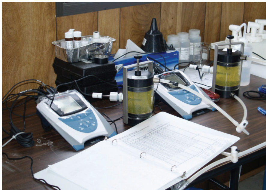
Figure 4.46: Serially Connected Flow Cells with Electrodes Connected to Digital Voltmeters
