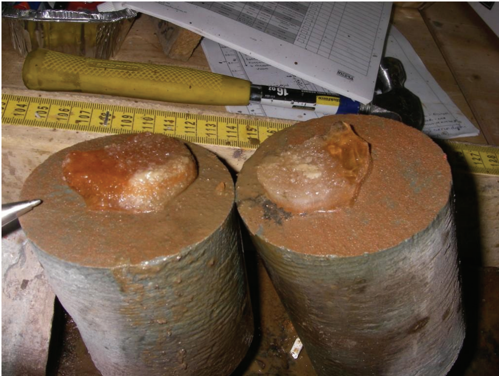
Figure 3.28: Halite-infilled Horizontal Fracture at 458.6 mBGS in Upper Queenston Formation in DGR-3
