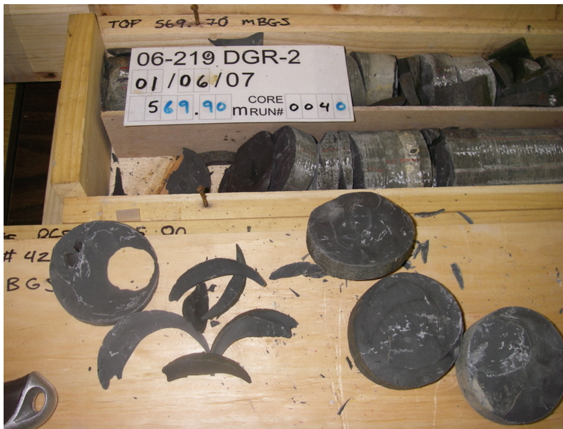
Figure 3.35: Core Disking in Upper Georgian Bay Formation Shale, 569.90 mBGS, DGR-2
