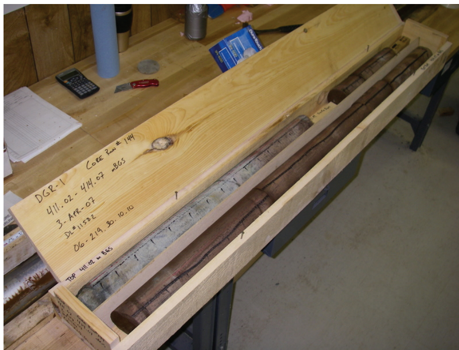
Figure 3.26: Top of Cabot Head Formation Shale, 411.02 to 414.07 mBGS in DGR-1
