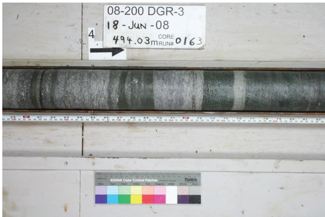
Figure 3.31: Interbedded Green Shale and Grey Fossiliferous Limestone, Middle Queenston Formation at 496 mBGS in DGR-3
