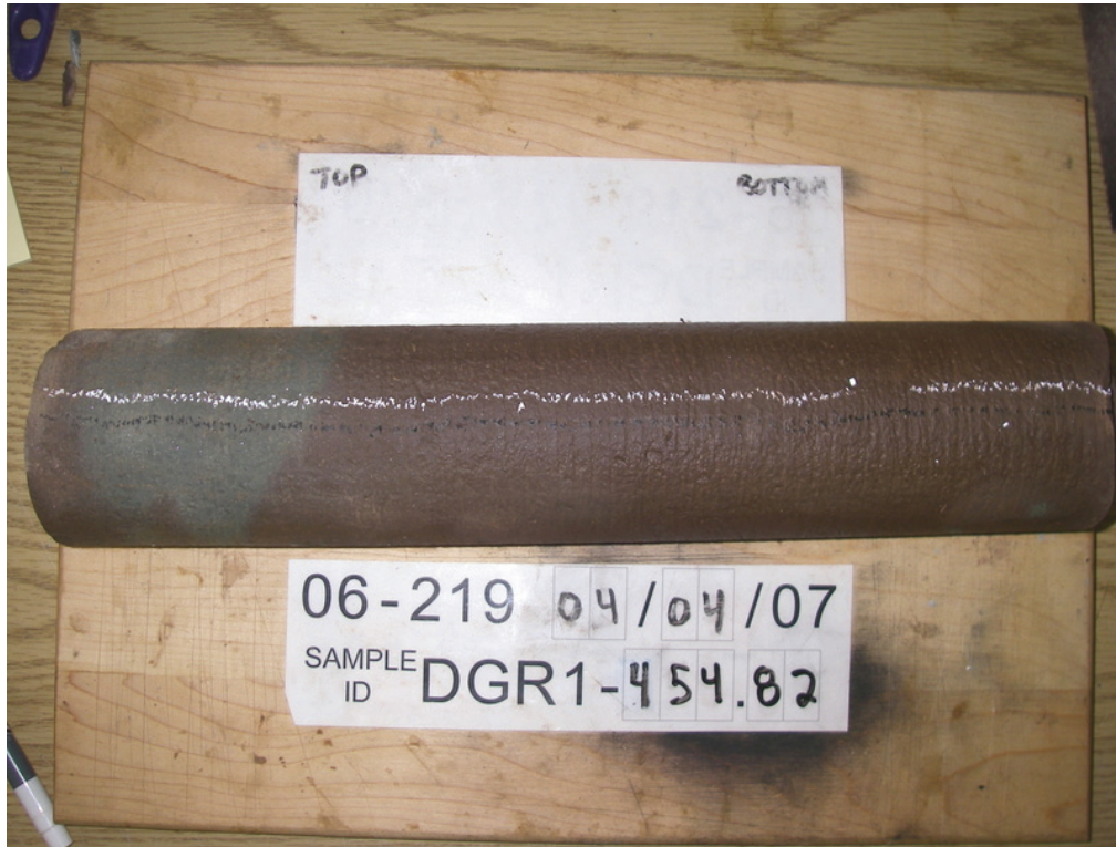
Figure 3.29: Core Sample of Green and Red Shale, Upper Queenston Formation, 454.82 mBGS, DGR-1
