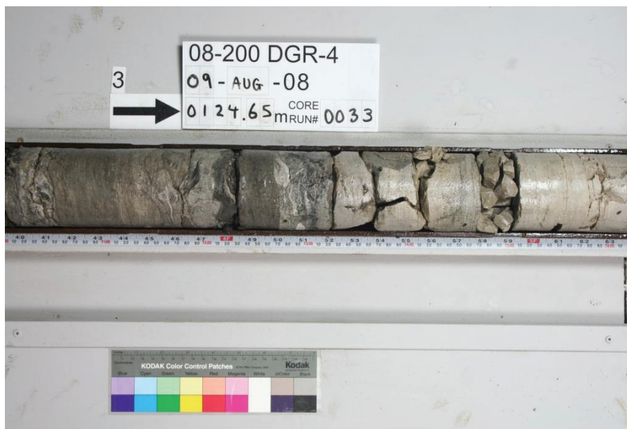
Figure 3.55: Devonian-Silurian Unconformity (Middle of Core Photo) at the Depth of 126.0 mBGS in DGR-4
