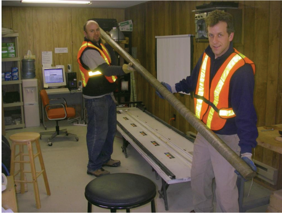
Figure 3.23: Intact 3.0-m-length Core of the Salina A0 Unit Dolostone at 371-374 mBGS in DGR-1
