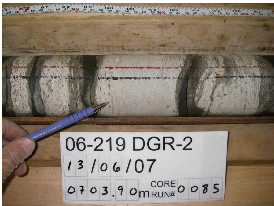
Figure 3.43: Core Sample of Lower Member of Sherman Fall Argillaceous Limestone, 703.90 mBGS, DGR-2
