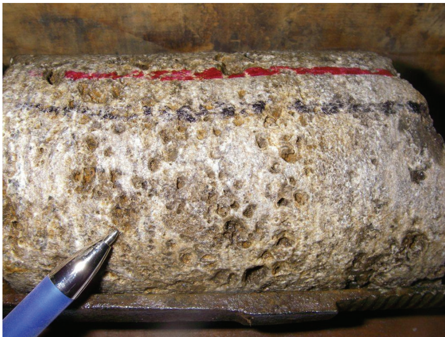
Figure 3.22: Open Vuggy Porosity of Upper A1 Unit Carbonate at 326.2 mBGS in DGR-4
