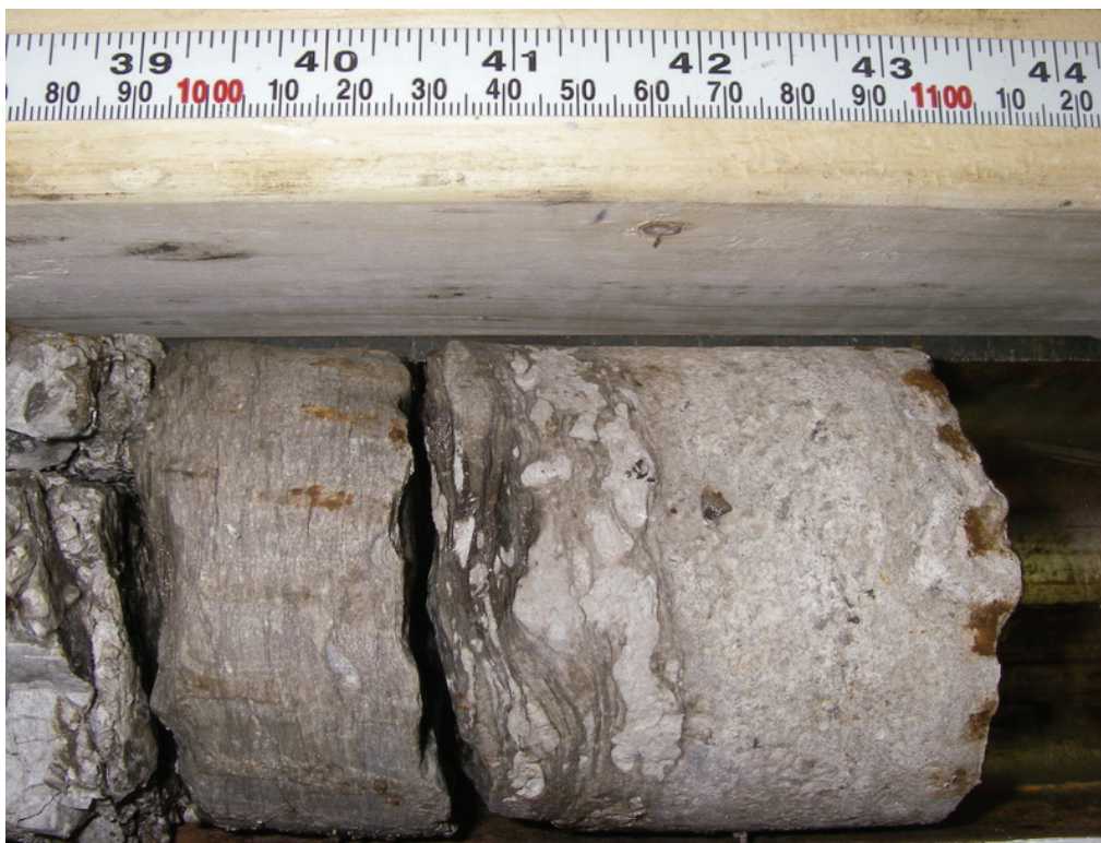
Figure 3.18: Core Sample of Bois Blanc Formation Cherty Dolostone with Bituminous Laminations, 102.3 mBGS, DGR-1
