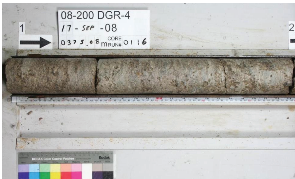
Figure 4.91: Permeable Vuggy Core in Guelph Formation Dolostone, 375 mBGS, DGR-4
