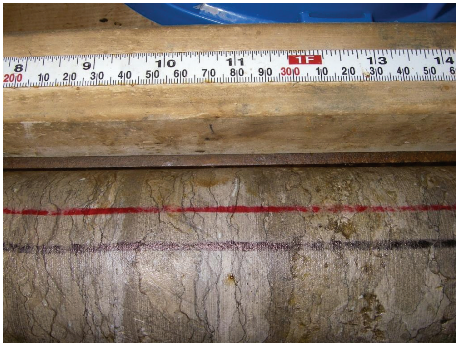
Figure 3.45: Trace of Hydrocarbon Weeping from Stylolites, Gull River Formation, 817.0 mBGS in DGR-2
