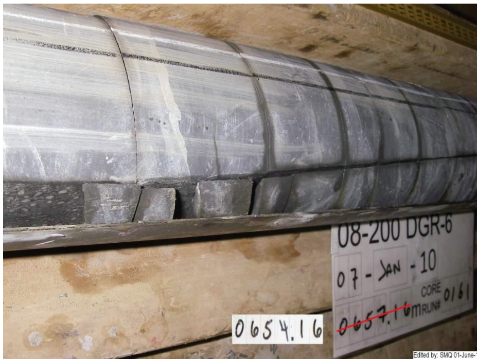
Figure 3.66: Inclined Halite-infilled Fracture at Depth of 655.3 mLBGS in Georgian Bay Formation, DGR-6
