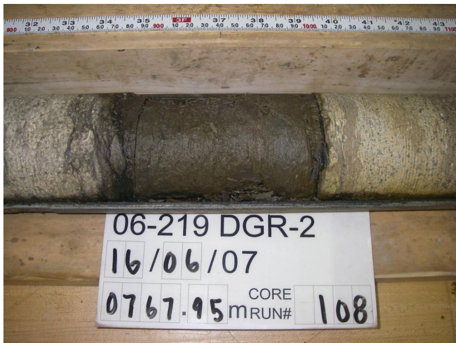
Figure 3.44: Volcanic Ash Bed, Coboconk Formation, 768.6 mBGS, DGR-2
