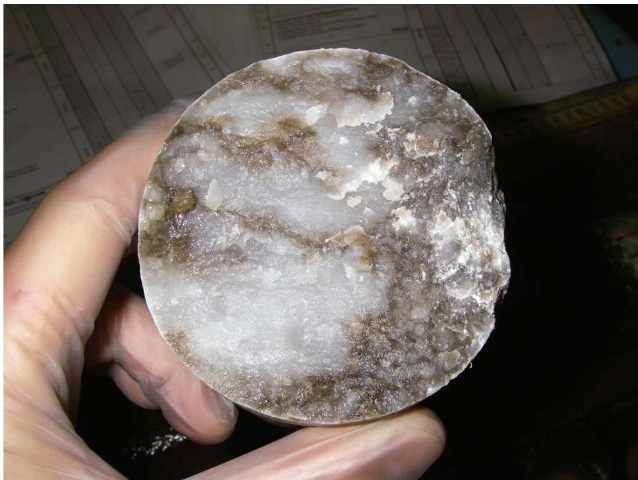
Figure 3.21: Dolomitic Anhydrite of Salina A2 Unit Evaporite, 322.75 mBGS in DGR-4
