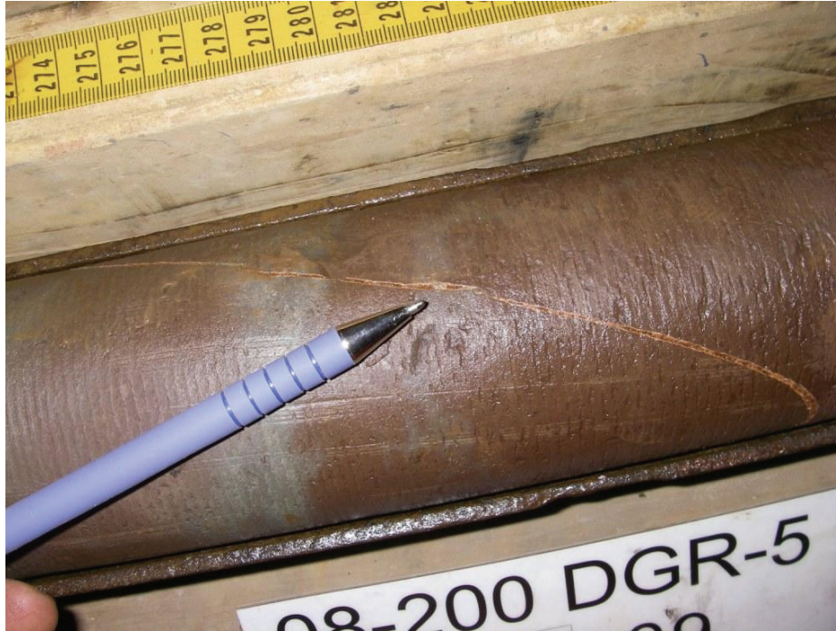
Figure 3.65: Inclined Halite and Calcite-infilled Fracture at Depth of 501.7 mLBGS in Queenston Formation, DGR-5
