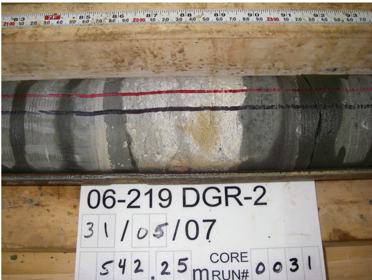
Figure 3.34: Core Sample of Upper Georgian Bay Formation Interbedded Shale and Limestone, 542.25 mBGS, DGR-2
