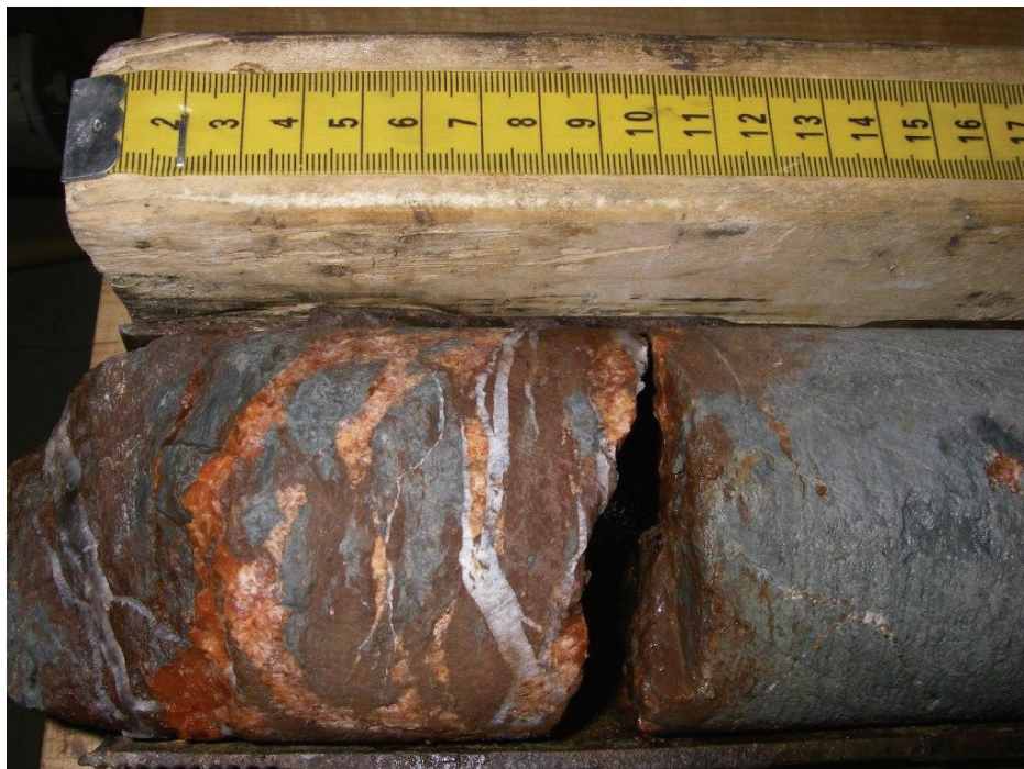
Figure 3.19: Orange Anhydrite Veins Cut by White Gypsum Veins in Salina F Unit Dolomitic Shale, 222.6 mBGS in DGR-3
