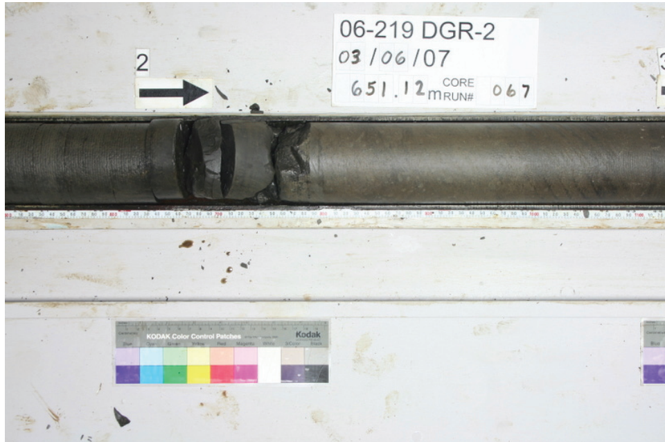
Figure 3.38: Contact between Dark Grey Blue Mountain Formation (Left) and Brownish-Grey Collingwood Member of the Cobourg Formation (Right), 651.6 mBGS in DGR-2
