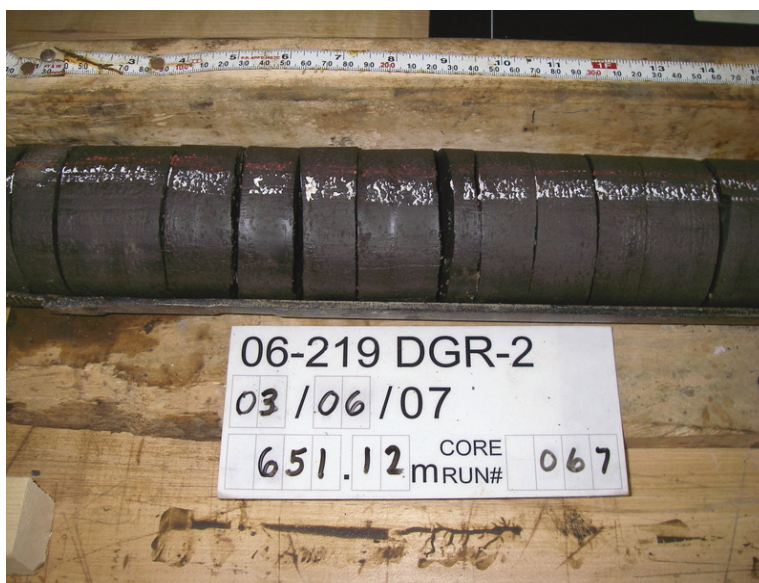
Figure 3.37: Core Disking of Lower Member, Blue Mountain Formation Shale, 652 mBGS, DGR-2
