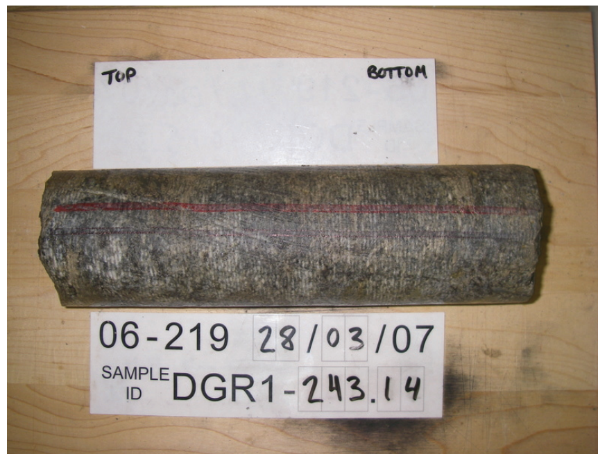
Figure 3.20: Core Sample of Salina D Unit Anhydritic Dolostone from 243.14 mBGS in DGR-1
